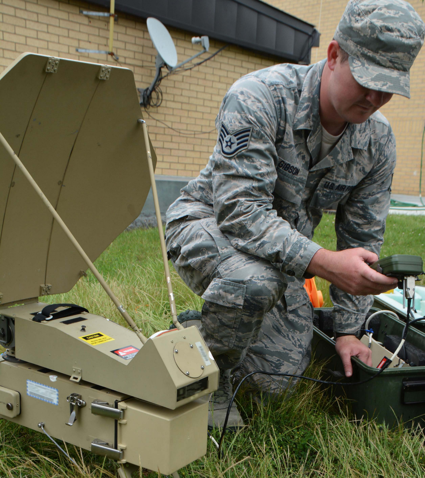
Staff Sgt. Colten Gibson of the 507th Air Refueling Wing Command Post configures a SCAMP (Single Channel Anti-Jam Man Portable) terminal during the June Operational Exercise at Tinker Air Force Base, Okla. The primary mission of SCAMP is to provide survivable extended-range communications to tactical units for command and control. (Photo by Tech. Sgt. Lauren Gleason)
